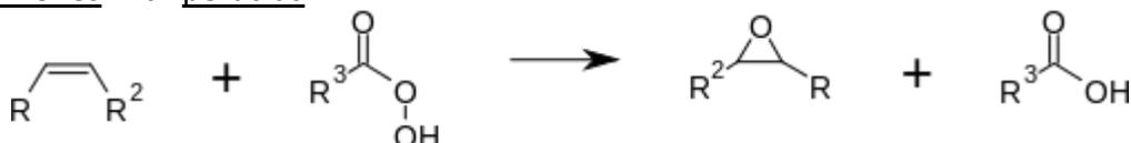
As can be seen, in contrast to glycidyl-based epoxy resins, this production of such epoxy monomers does not require an acidic hydrogen atom but an aliphatic double bond.
