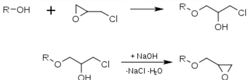
First a hydroxy group reacts in a coupling reaction with epichlorohydrin, followed by dehydrohalogenation.
