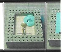
7. This type of silicone rubber has to cure overnight. When cured, peel the insta-mold off of the back. Leave the mold in the lego blocks for the moment.
