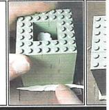
4. When dry, remove the legos from around the mold and snap the plexiglass off. the mold should look something like this.
